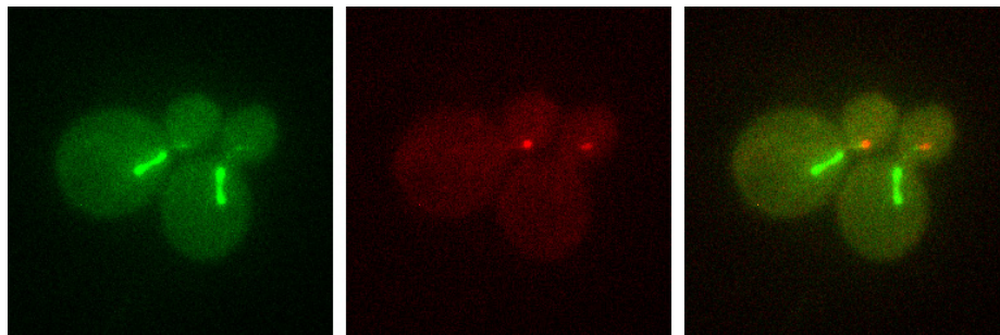
Figure 2: “Zero pixel shift” enables accurate interpretation of biological data. In this example tubulin was labeled with CFP and karyogamy protein was labeled with YFP in yeast cells, and the images of the two fluorophores were acquired using “zero pixel shift” filter sets mounted in a Carl Zeiss microscope equipped with a 100x, 1.45 NA objective. There is almost no pixel shift between CFP (green) and YFP (red) images, as evidenced by the fact that karyogamy protein clearly appears at the very tip of the microtubule in the merged image (c). Images courtesy of Mohan Gupta and David Pellman at Dana-Farber Cancer Institute and Harvard Medical School in Boston.
