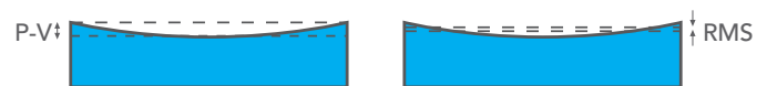
Figure 1. Flatness as measured by the peak to valley method (P-V) vs RMS flatness.
